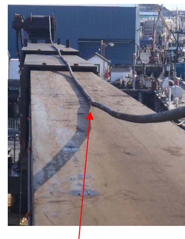
Figure 6 – Note abnormal bend in wire where stored.
